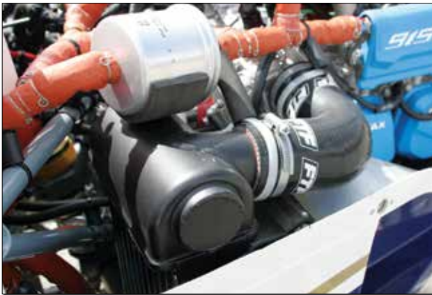
The intercooler is large, providing significant cooling after the turbocharger compresses the air, making for better efficiency and more power.
