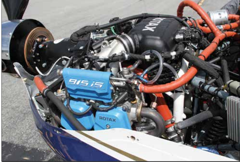
The turbocharged Rotax 915 iS fits nicely under the cowling of the TSi and provides plenty of power.
