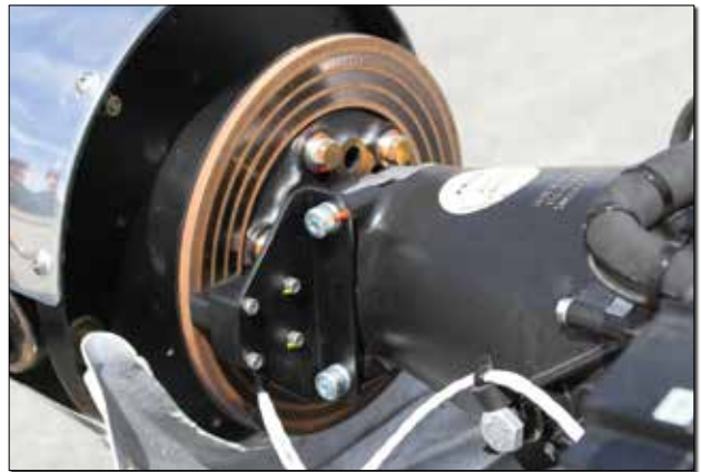
The slip ring on the rear of the Airmaster prop provides power and control for the electric constant-speed blades. It's a good match for the 915 iS engine.
