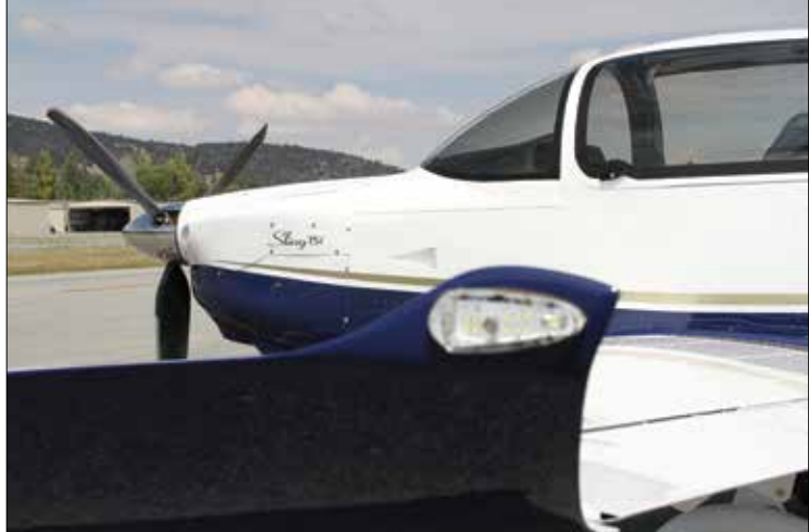
(Left) The wing tips on the all-new wing are actually small winglets. (Right) The wing design is all new on the TSi, sharing almost no parts with the Sling 4. The winglet tips make for an excellent high-altitude cruising machine.
