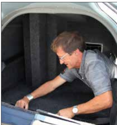
(Left) Folding the rear seat back down creates a cavernous baggage compartment, and the baggage door is big enough to crawl through, making loading and unloading easy. The vertical column is the housing for the optional whole-airframe ballistic parachute. (Center) The TSi has an optional ski tube that is good for long, lightweight items. (Right) Want to camp with your airplane, but hate tents? Install the optional ski tube, fold the rear seats down, and you've got a camper!
