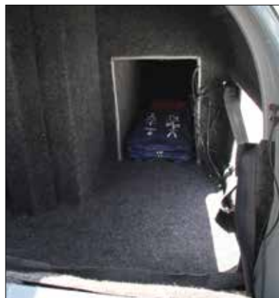
(Left) Folding the rear seat back down creates a cavernous baggage compartment, and the baggage door is big enough to crawl through, making loading and unloading easy. The vertical column is the housing for the optional whole-airframe ballistic parachute. (Center) The TSi has an optional ski tube that is good for long, lightweight items. (Right) Want to camp with your airplane, but hate tents? Install the optional ski tube, fold the rear seats down, and you've got a camper!
