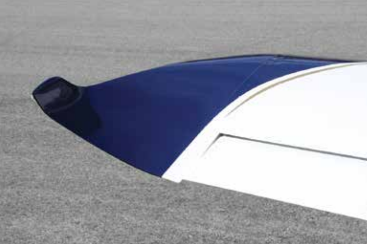
(Left) The wing tips on the all-new wing are actually small winglets. (Right) The wing design is all new on the TSi, sharing almost no parts with the Sling 4. The winglet tips make for an excellent high-altitude cruising machine.
