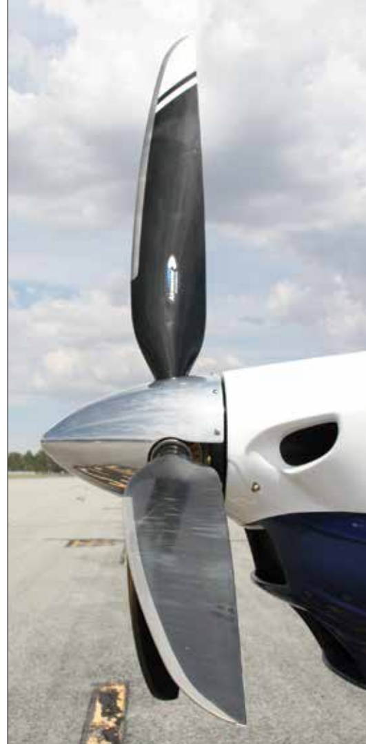
(Above) The large NACA duct on the right side of the cowling is for the intercooler. (Right) The Airmaster constant-speed prop is fitted with WhirlWind blades.
