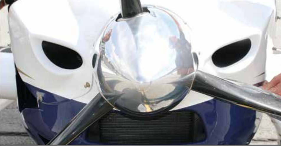
(Above) The large NACA duct on the right side of the cowling is for the intercooler. (Right) The Airmaster constant-speed prop is fitted with WhirlWind blades.
