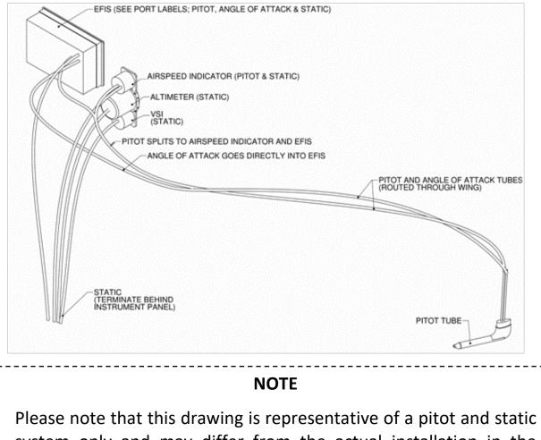
Please note that this drawing is representative of a pitot and static system only and may differ from the actual installation in the aircraft. For example, placement of instruments and actual instruments installed.
